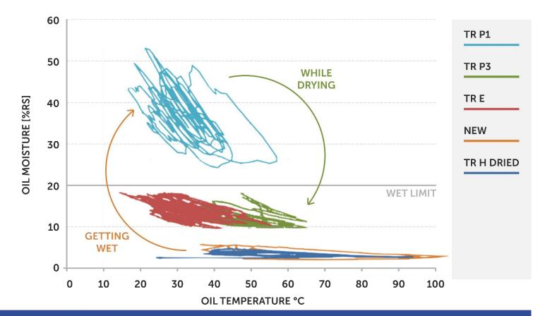
FIGURE 5.29 HYSTERESIS LOOPS PF %RS VS TEMPERATURE IN TRANSFORMETS WITH DIFFERENT MOISTURE
