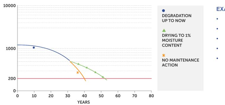
PAPER DEGRADATION SIMULATION WITH STABLE LOAD (TEMPERATURE)
