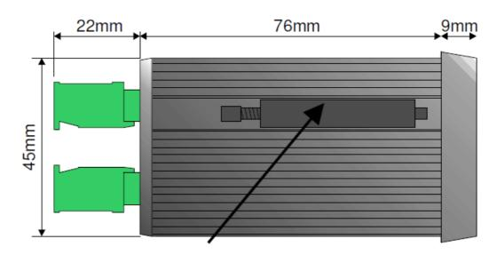
Fitting the retaining clip and screw (after the unit has been placed in the panel).
