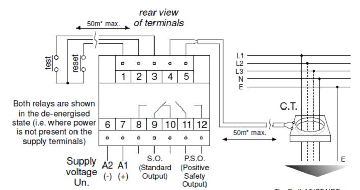
The Earth MUST NOT pass through the C.T. For single phase applications, only the live and neutral need to be passed through the C.T. \*Cabling:
