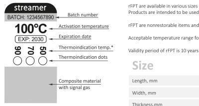
\*When the contact/cable is heated above the thermoindication temperature, the dot irreversibly changes its color to black
