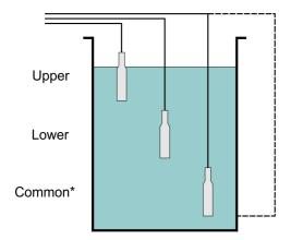
\*Common probe not required if tank/container conductive. Connection from Level controller can then be made directly as shown by the dashed line.
