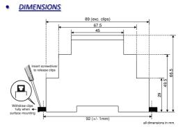
On to 35mm symmetric DIN rail to BS EN 60715 or direct surface mounting via 2 x M3.5 or 4BA screws using the black clips provided
